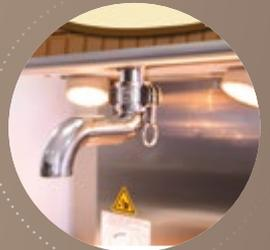
Equipped with stainless steel tap easy to be adjusted to supply the arc diffuser to do the total enrobing.
