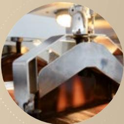
The «Easy Cut System» allows for a quick and easy paper cut avoiding any slowdown in the couverture cycle or damage to the coating belt.
